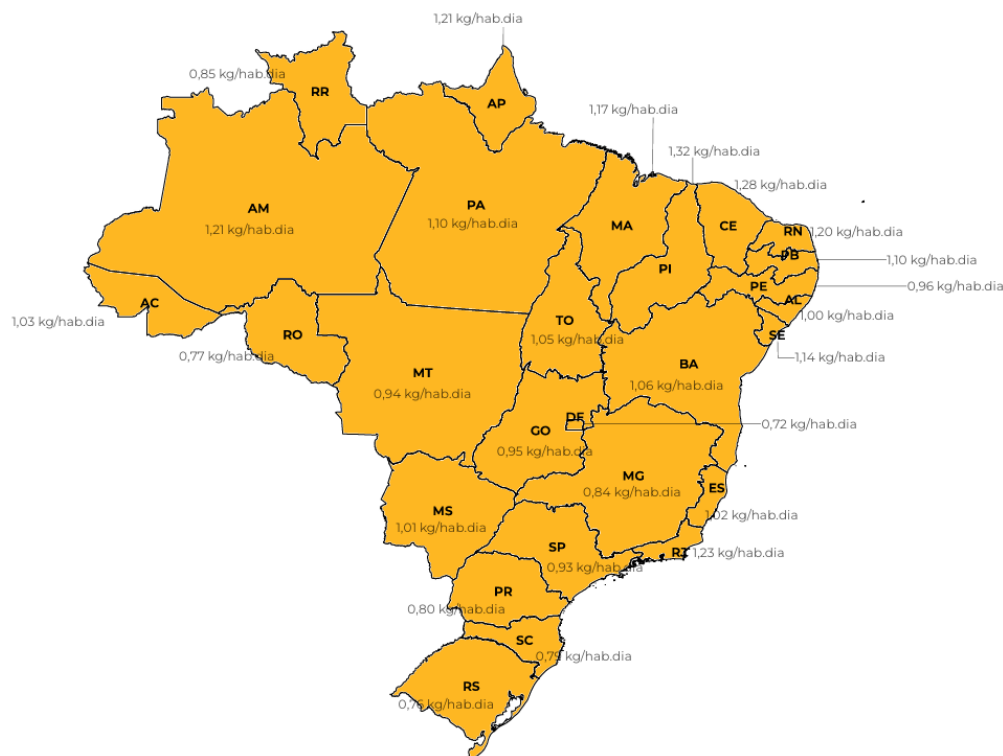
Figure5 - Per capita MSW collected relative to the total population served by state (in kg/capita/day/state, in 2022). Source: Ministry of Cities (2023).
