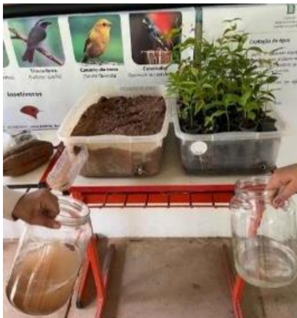
Figure 6- Test simulating the effect of rain on degraded and non-degraded soil to observe water infiltration. Source: Author (2023).
