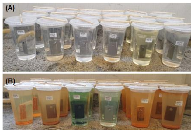
Figure 5 - Corrosion test: (A) start of the test; (B) after 21 days of testing. Source: research data
