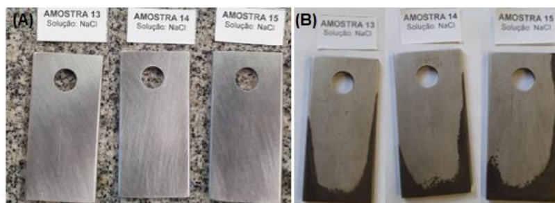
Figure 21 - Color specimen used in the test in NaCl solution without inhibitor: (A) before the test; (B) after 21 days of testing. Source: research data
