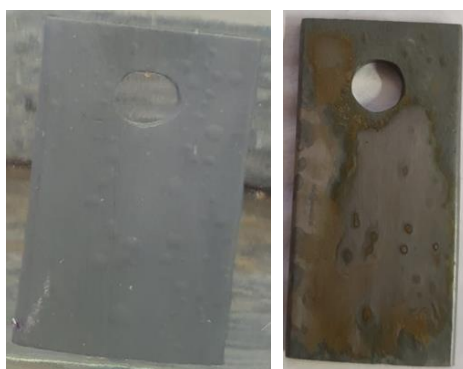
Figure 16 - Corrosion by Hydrogen Blistering. Source: research data
