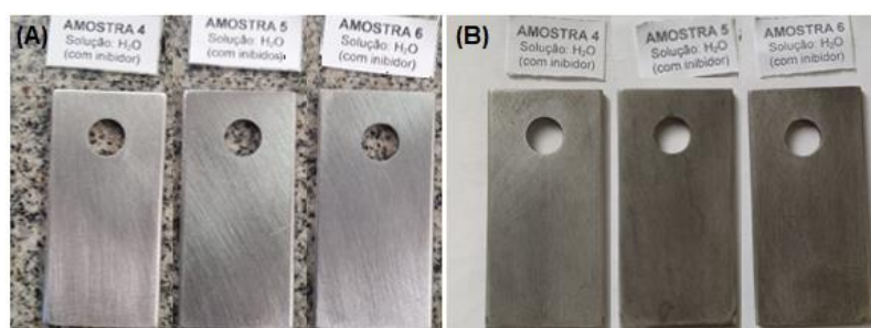
Figure 13 - Specimen used in the test in H_2O solution with inhibitor: (A) before the test; (B) after 21 days of testing. Source: research data
